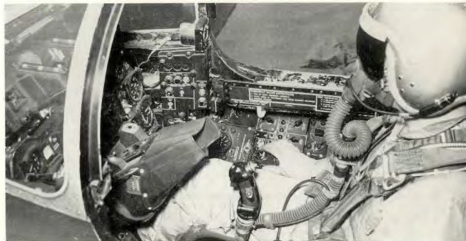
Above, control box, as installed in F-86D. Below, pilot demonstrates fingertip control.
