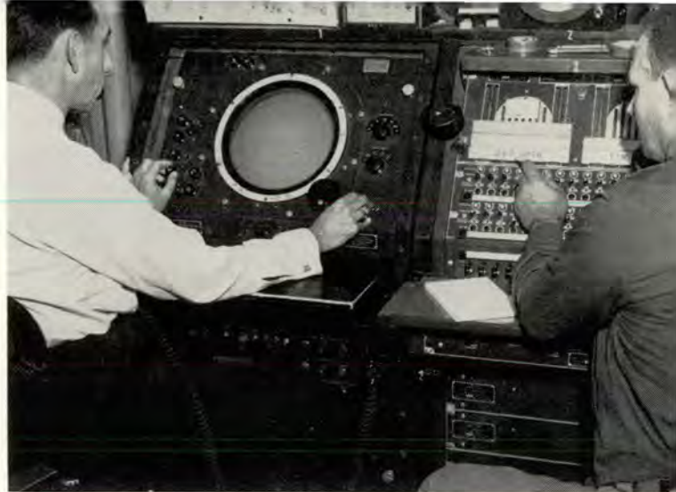
From flight data position, clearance is given to pilot over one of 22 radio frequency channels available. Operator gives vector headings to departing aircraft as coordinator keeps tab on other planes in area.
