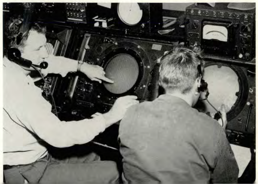
Feeder controller, left, turns over aircraft to the precision approach radar operator for landing.
