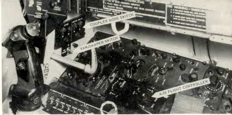
Above, control box, as installed in F-86D. Below, pilot demonstrates fingertip control.
